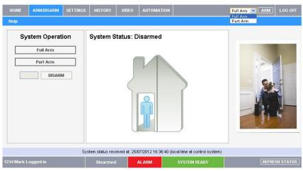
Set and unset the system using the System Operation Area buttons or upper-right Set button (with Full Set/Part Set dropdown).
