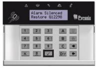
When the time is displayed, enter the number given to you by the ARC. 'Engineer Reset Performed' will be displayed. Press the 🗴 key to back to the time.
